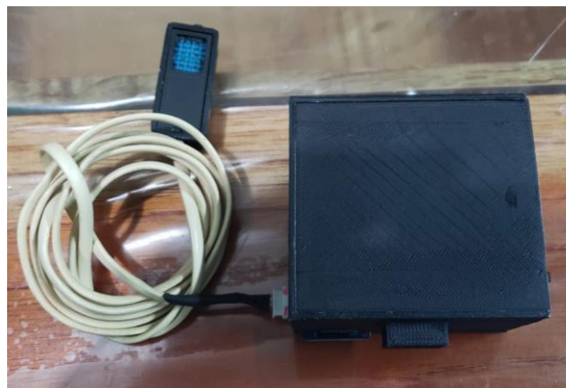
Figure 2.4 Thermometer installed to measure wall internal and external air temperature at Monterreal houses.
