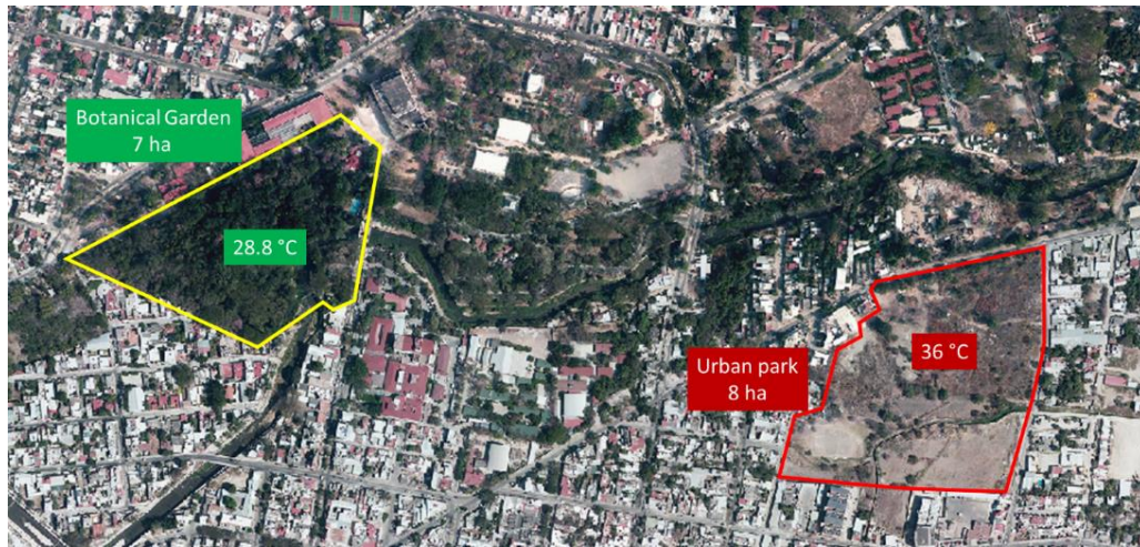
Figure 1.9 Comparison of land surface temperature (LST) registered at two contiguous woodland areas with different tree density.
