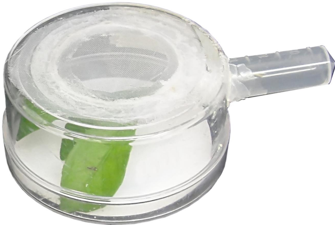
Figure 4.1: Arena used for inoculation of D. citri adults and nymphs (Image Valdez-Carrasco, 2016).
