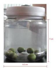
**Figure 3.1**. Flask used to evaluate respiration rate and ethylene production in coffee fruit during storage inside biodegradable bags at  $4 \pm 1$ ,  $8 \pm 1$  and  $24 \pm 3$  °C for 28 days.
